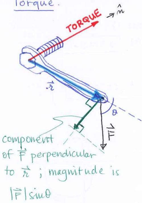
TORQUE VECTOR when we use  $\vec{F}$  force to turn a bolt, applied  $\vec{r}$  away from the bolt's head, is:
