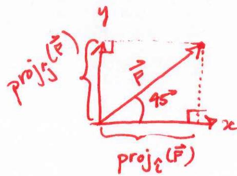
The VECTOR PROJEC'N of  $\vec{u}$  onto  $\vec{v}$  ( $\neq \vec{0}$ ) is the vector determined by dropping a perpendicular line segment from the head of  $\vec{u}$  onto  $\vec{v}$ .
