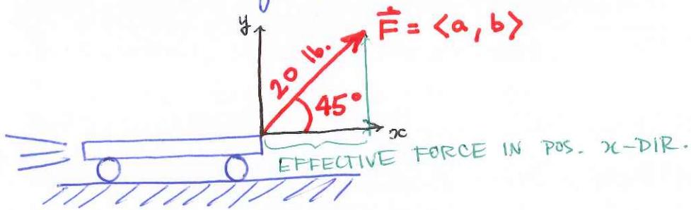
The effective force moving the cart forward is just the x-component of  $\vec{F}$ . In our diagram, that's a.
